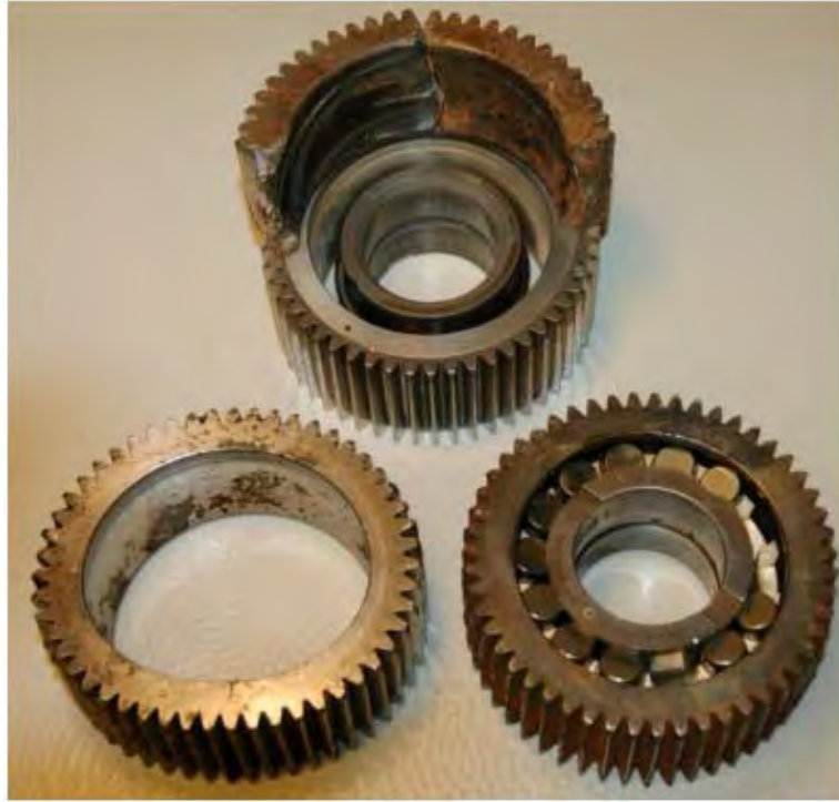
Picture 1. Fractured Planet Gear (Top Center) (AIBN June 28 Report at 3)
