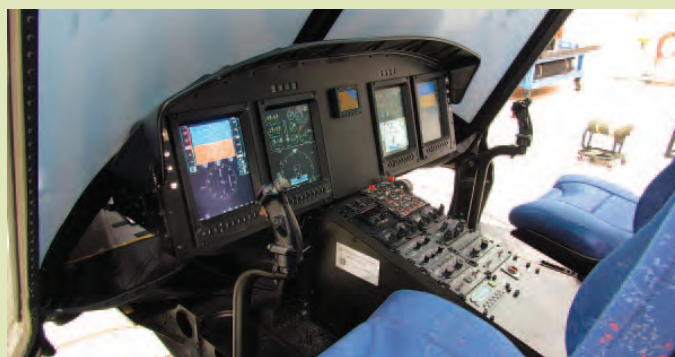
Vector Aerospace has selected 10-inch Sagem displays for its integrated digital cockpit retrofit for the Bell Huey UH-1H.
