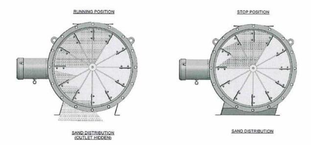
The Product is a rotating paddle wheel inside of a drum with an inlet and outlet sized to measure a determined amount of material.
