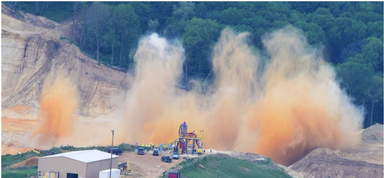
Example of blasting operations at a Wisconsin frac sand mine, with silica dust hurled into the air.
